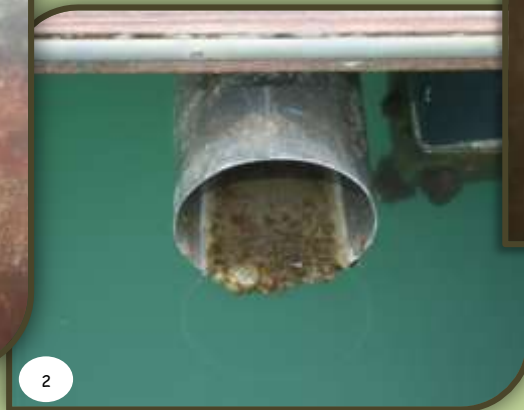
Photo 2: Bladder weed ( Colpomenia spp.) fouling the engine exhaust of a recreational vessel.
